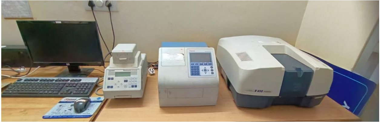
Desktop with softwares of the instruments, ELISA, UV spectrophotometer, Left to right : Thermocycler , ELISA reader, UV spectrophotometer (JASCO-JAPAN)
